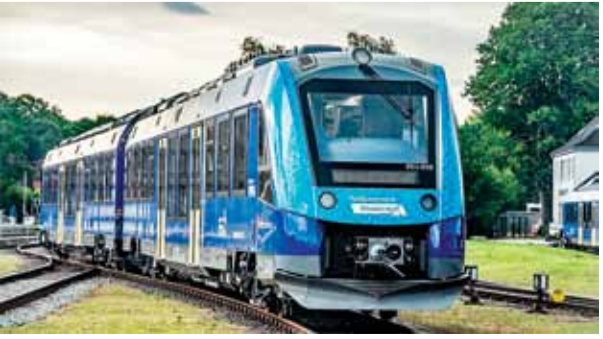
Hydrogen-powered trains generate electricity through fuel cells by combining hydrogen and oxygen, with water being
