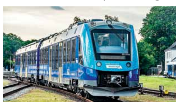
Hydrogen-powered trains generate electricity through fuel cells by combining hydrogen and oxygen, with water being
